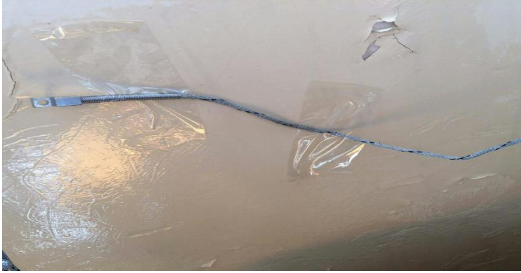
Figure 6. Thermocouples measured inside surface temperature
