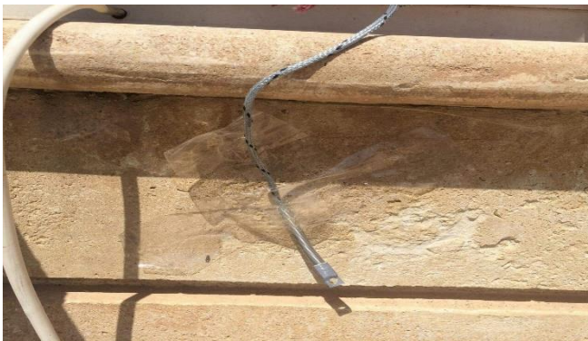
Figure 5. Thermocouples measured ambient and outside temperature
