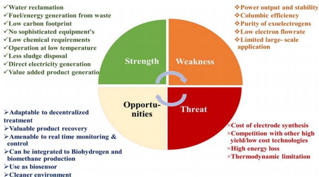
Figure 4. Schematic representation of the strength, weakness, opportunity, and threat of MES system (Koroglu et al. 2019; Kumar, Agrawal, and Verma 2021)
